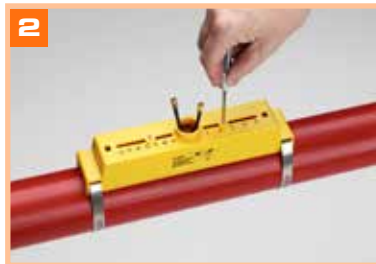
Clamp guide rail and sensor assembly to pipe and release sensor locking screws after adjustment
